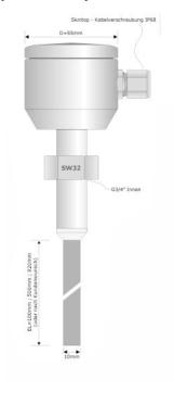
Please note that during installation and removal of coated probes, the coating is not damaged. Damage can lead to errors in the evaluation!
